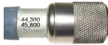
Base of flex aerial with engraved frequency range.
