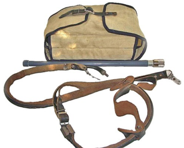
Quince radio packed for transit with flex aerial and shoulder strap aerial.
