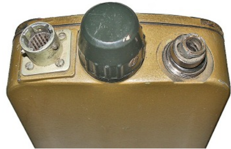
Top view showing remote control socket, channel and volume control, and aerial socket.
