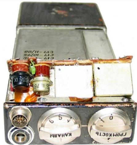
Internal view of top section Angstrom CH, showing controls, aerial socket and remote control socket.
