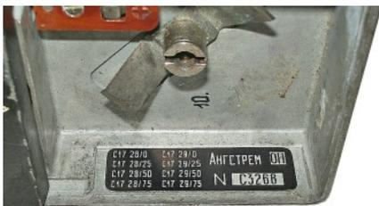
Battery compartment with serial and type number plate showing channel numbers.
