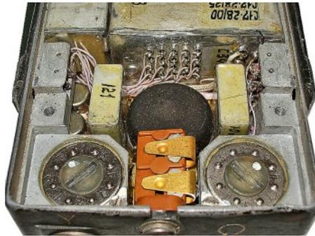
Internal view of top section Angstrom OH showing the two controls and earphone socket.
