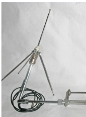
Lily receiver with associated flexible wire aerial and remote control unit.
