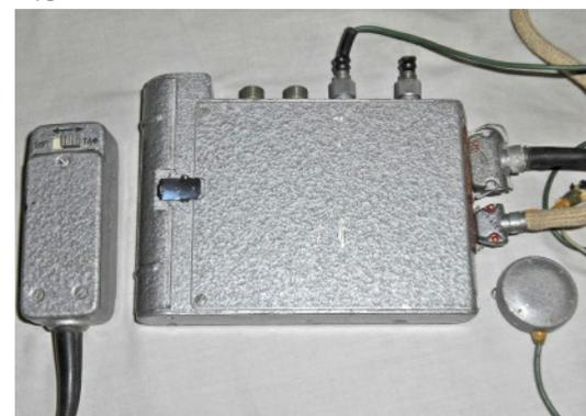
Rear view of a Kopchik receiver and associated remote control unit. Note a CW-FM/AM mode switch at the back of the remote control unit.
