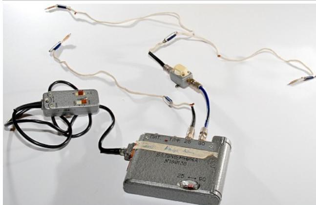
Kopchik receiver with remote control unit and two different wire aerials. Note a small attenuator box in the dipole feeder which was used when limited DF function was required.
