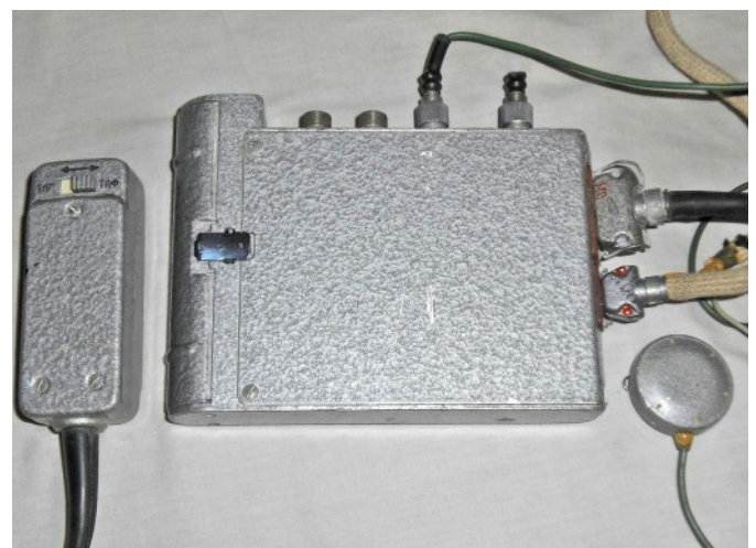
Rear view of the Kopchik receiver and associated remote control unit.
