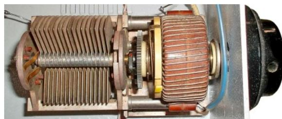
Detail view of 'T' aerial matching section of the Systema R transmitter. One rotation of the capacitor (W) automatically engaged one tap up- or downwards on the coil. This could also be done manually by a switch (Z).
