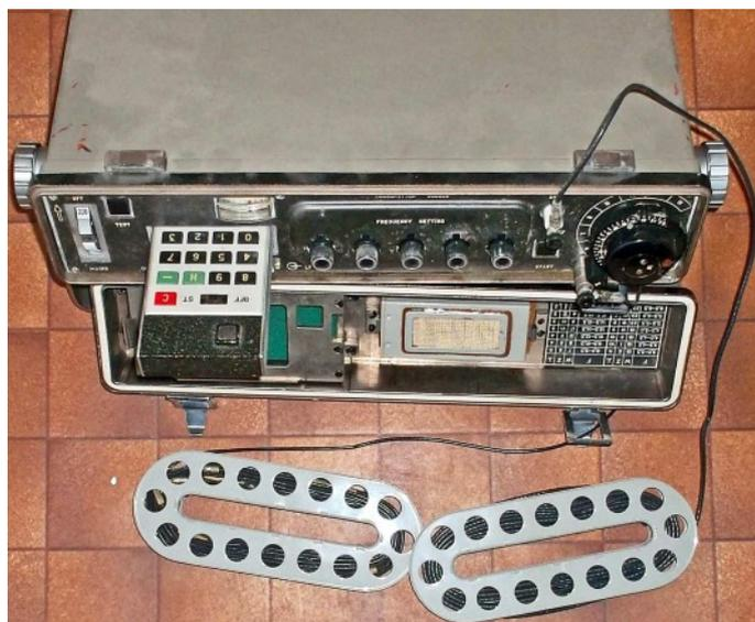
View of Systema R transmitter showing the encoder/keyer in position, when not in use it was stowed in the cover (top picture). Note the aerial and counterpoise on spools.
