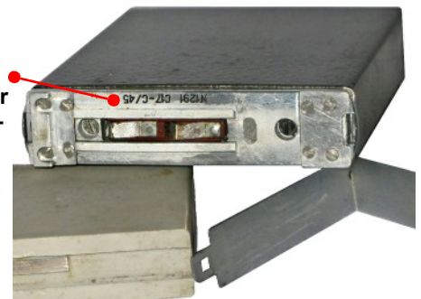
Bottom view of Orange-2 showing battery contacts, battery and battery retaining clip.
