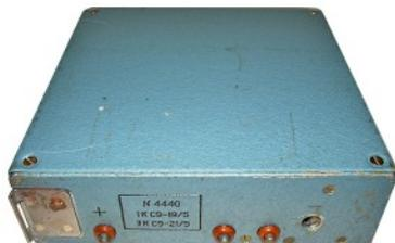
Bottom view of Ataka showing battery contacts and fixing arrangements. The set had a die-cast aluminium alloy frame.
