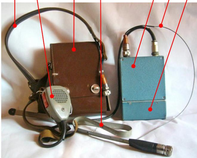
Ataka in a leather carrying case with aerials and combined speaker-microphone. The latter had a channel switch, volume control with on/off switch, PTT button, and two tone buttons.
