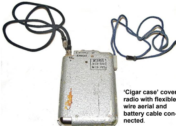
'Cigar case' covert radio with flexible wire aerial and battery cable connected.
