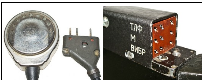
Covert speaker (left) ; 3-pt plug (centre), and socket panel for connecting speaker, microphone and vibrator.
