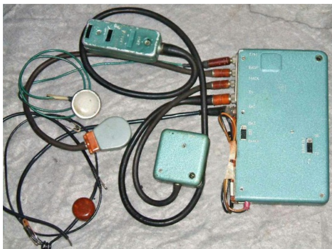
Anker with accessories, but less the battery pack which would slide to the left hand side of the main body, connected by the two cables coming from the bottom side.
