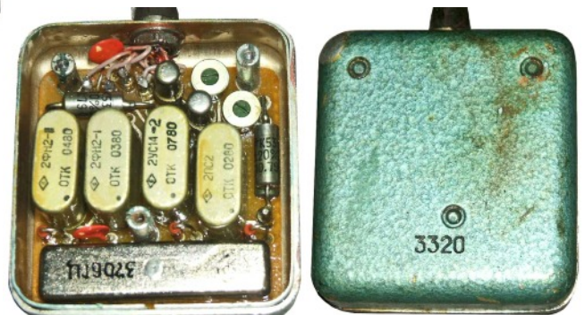
Internal view of components and bottom view of the external speech masking (scrambler) unit.
