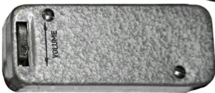
Back view of single channel remote control unit used with Kama 1 channel model.
