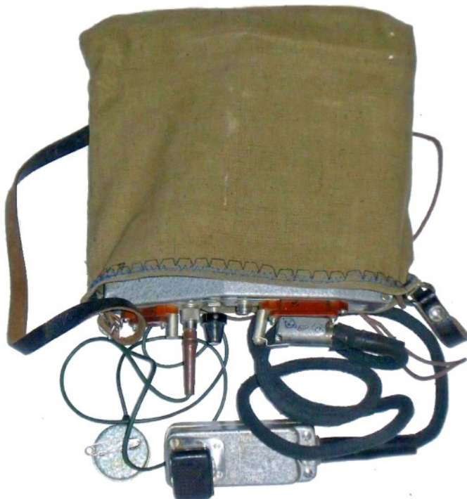
Kama variation 'A' single channel model in a canvas carrying bag, worn on the chest.
