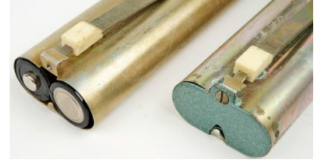
Detail view of battery holder which took 6 standard AA dry batteries or rechargeable NiCad batteries.
