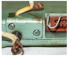
Close up view of of remote control unit socket and plug. Note the permanently attached microphone/speaker, aerial and counterpoise leads. (Serie AM)
