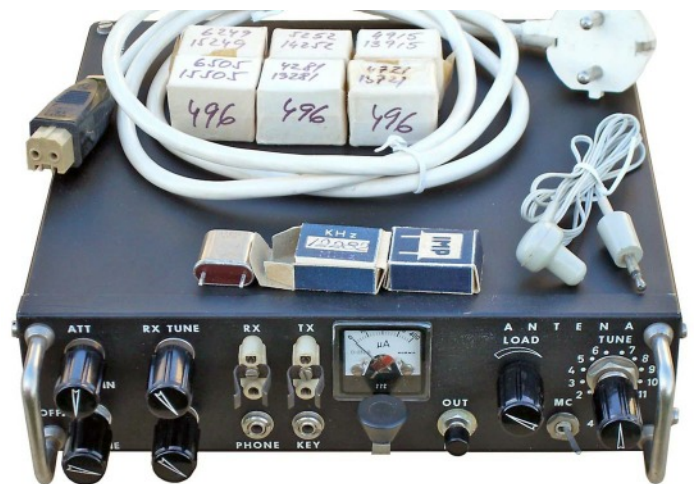
General view of the RTP8-SSB with associated accessories. Note 9MHz shift in the frequencies of the 6 sets of crystals on top of the set.
