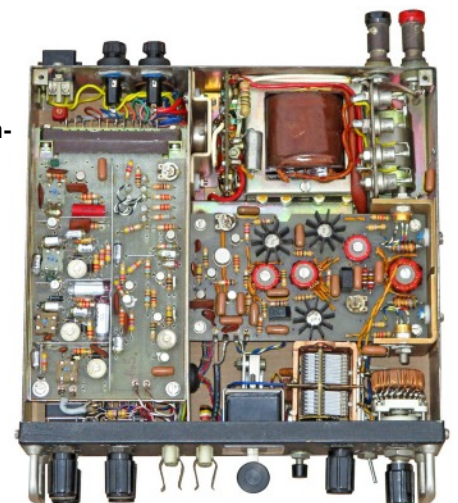
General view of the RTP8-SSB with associated accessories. Note 9MHz shift in the frequencies of the 6 sets of crystals on top of the set.
