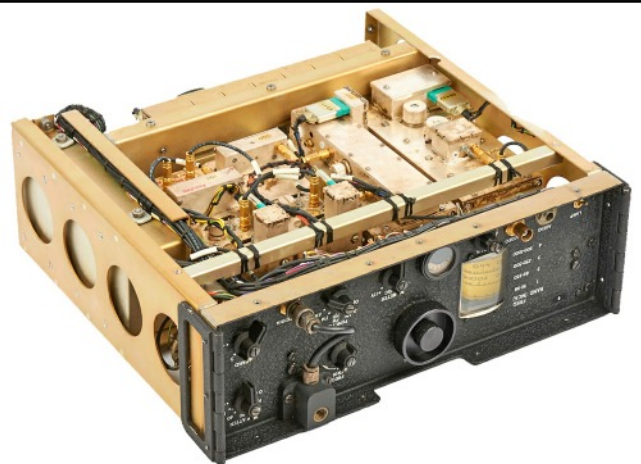
Bottom view of Radio Receiver SRR-8 showing the tuner assembly that housed four separate RF tuners.
