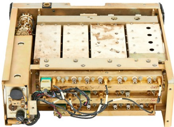
Top/rear view of SRR-8 with cover removed. Mounted at the rear were a 25 MHz IF strip with video detector; a 6 MHz IF strip with AM and FM detector, and AF amplifier.
