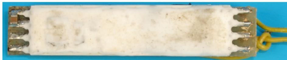
Underside circuit board 33014 showing a thick film module.
