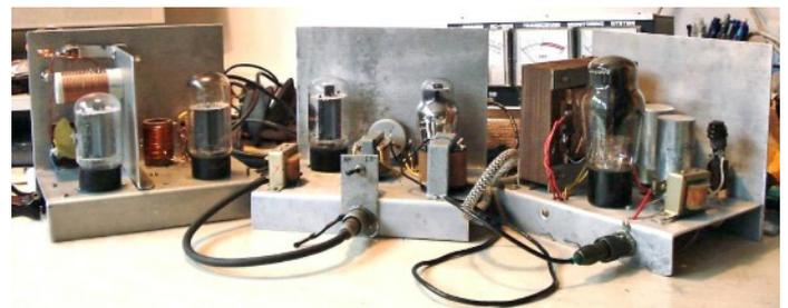
Chassis view of a replica Kričač transmitter unit (left), modulator unit (centre) and mains power unit (right), constructed by Janez Červek.
