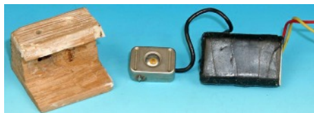
Unknown NF-B bug, with a separate Sennheiser microphone, used in the Rumelsburg prison. The microphone was hidden in a wooden dowel above the cell door.
