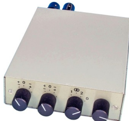
Line amplifier 33406-13, was used for monitoring two different microphones, or two microphones installed in one Operation Object for stereo listening.
