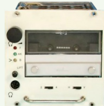
CAG-A (German A = Aufnahme = recording) compact cassette recorder for rack mounting which was used for recording intercepted messages after 1980 (above) and successor CAW-E (German E = Einschub = plug-in to EGS-System). (below)
