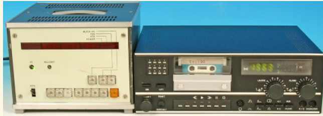
Evaluation equipment with a single cassette deck CAW-W (German W = Wiedergabe = playback) and AT3 evaluation unit (left).
