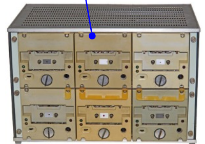
MTG tape recorder frame with 5+1 CAG-A compact cassette recorders for 5 Operational Objects plus one spare.
