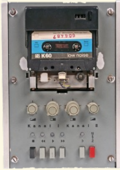
Earlier evaluation desk equipment CWG (Cassette Wiedergabegerät = cassette playback unit) and an AT2 evaluation unit (below).
