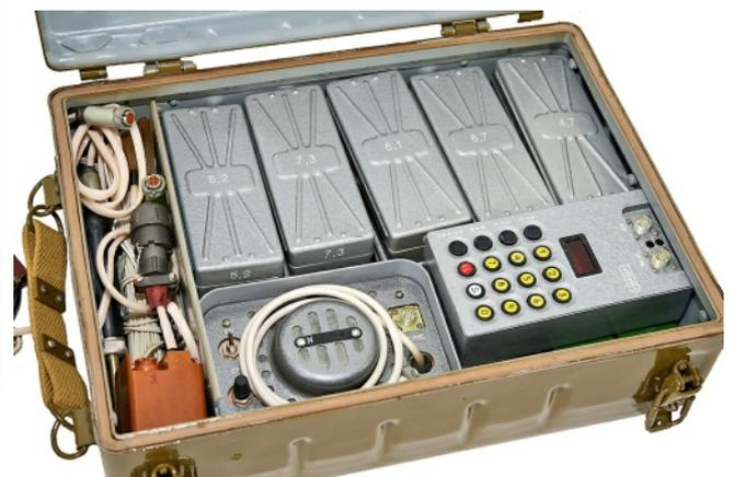
Severok K packed in metal unit transport case. For operational use in the field the loudspeaker and most of the plug-in RF units were not required.
