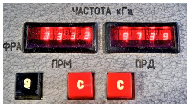
Detail view of receiver and transmitter frequency display
