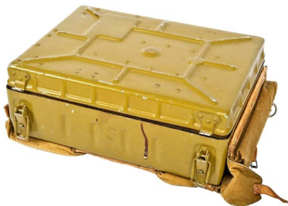
R-394 K with top cover closed forming a backpack harness.
