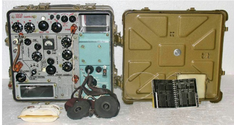
Front panel view of R-393, believed the B version without high speed Morse keyer.
