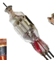
Philips EA 50 signal diode used as HT rectifier.
