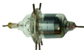
Philips E1F valve, equivalent to 954.
