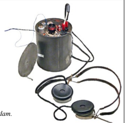
Clandestine midget receiver hidden in a pipe tobacco tin (#4B) constructed by a Philips employee. The receiver was built with two E1F valves, a metal rectifier, and a re-wound miniature loudspeaker transformer providing LT.
