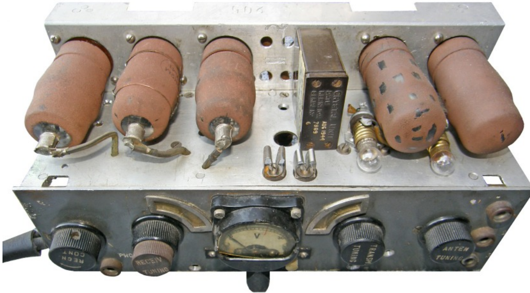
Transmitter-receiver chassis removed from its enclosure showing the front panel and positions of valves. Note the two contacts in front of the crystal leading via knife contacts to the Morse Key on the hinged top.
