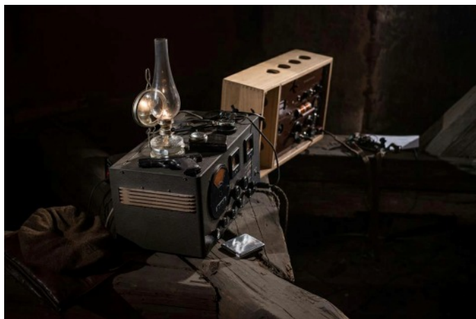
Hallicrafters SX 24 Skyrider Defiant receiver (left) and replica Mk.VI 'Libuše' transmitter (right) setup in April 2017. Permission was granted to transmit under the special temporary amateur radio call sign OL75SILVERA at a location originally used by the Silver-A group in 1942.
