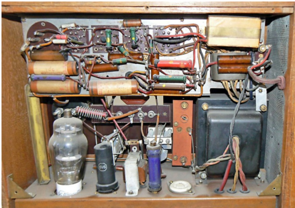
Rear view of a Mk.VI variation 1c suitcase transmitter. When taking this photograph the transmitter rectifier valve 5Z4 (right-empty valve holder-) was temporary removed in order to obtain an unobstructed view.
