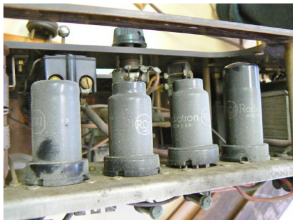
Side view of receiver section with 3 receiver valves and the rectifier valve at the right.
