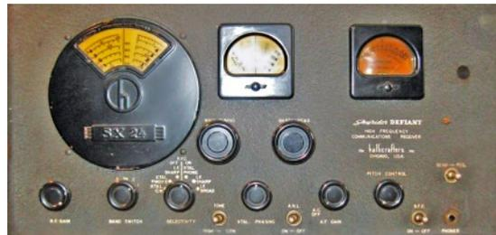
A commercial Hallicrafters SX 24 Skyrider Defiant was used by the Silver-A group as a replacement for the original Mk.VI 'Libuše' receiver, which was unsuitable for the task.
