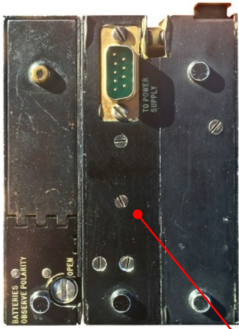
Bottom view of LP modules which were clipped on power unit module. (Low power version)
