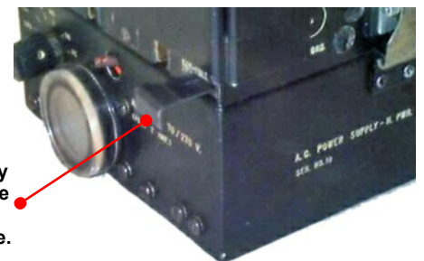
Detail view of AC mains power unit. Note the Morse key pullout lever on the bottom side of the transmitter module.
