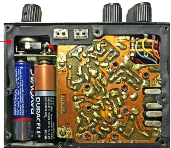
Receiver module, both sides shown.
