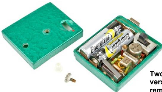
Two variations of the initial version of the transmitter remote control unit using two AA batteries.
