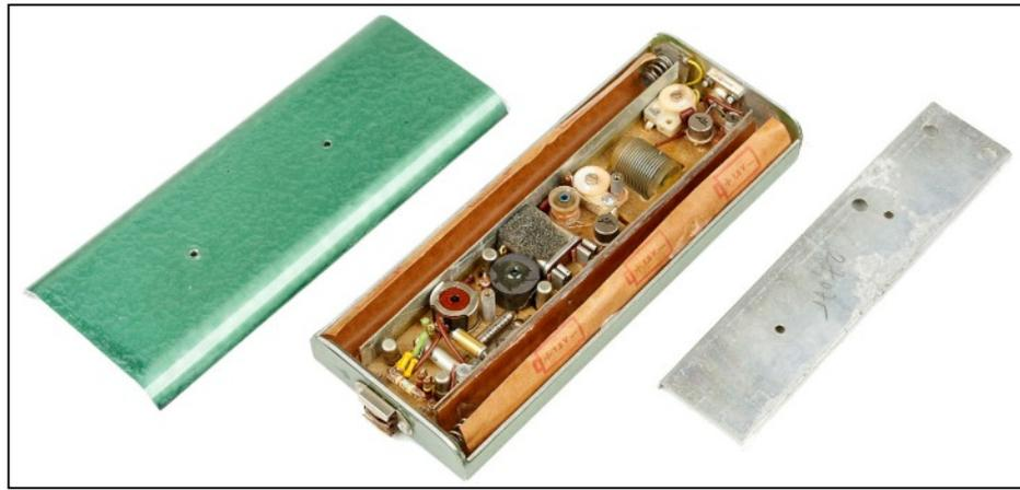
Internal view of two variations of the 'Poplach' transmitter unit: an earlier produced (left) and a later built transmitter which had a green hammer tone enclosure. Stacks of three AA batteries were placed on each side of the transmitter board inside the enclosure.
