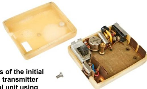
A later version transmitter remote control unit. It was powered by the transmitter batteries.
