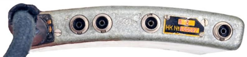
Bottom view of the Neva transmitter-receiver unit showing sockets for battery, earphone, vibrator and microphone. Note the slightly curved shape for carrying the set on the chest.
