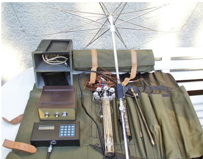
High speed keyer 32843 was principally used with transmitter WSA 6 of system 32240, here seen with an umbrella aerial and transit/storage containers.
