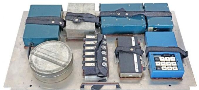
WSA 1 transmitter and associated equipment of system 32210 included an unknown high speed keyer (bottom right), which could be substituted by keyer 32843.
