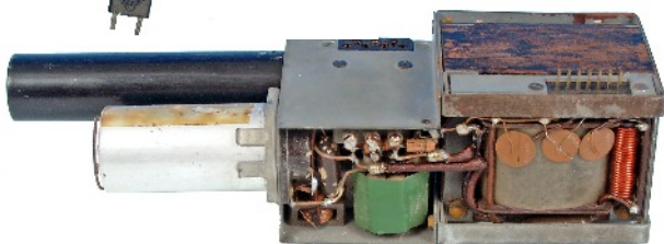
Combined AC/DC power unit which plugged into a socket located at the rear of the transmitter unit.
