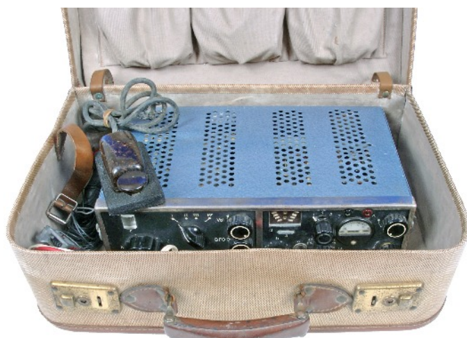
'Unknown SEL' agents set with ancillaries photographed in a 'period' suitcase, most probably not original.
