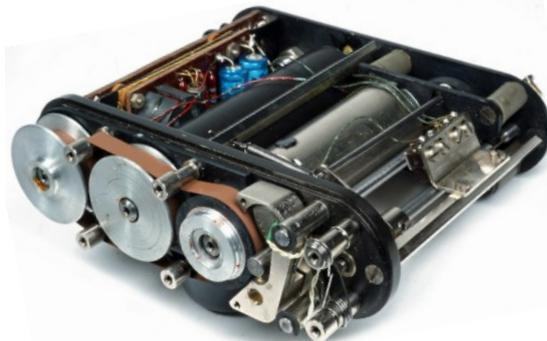
Top and side view of the tape recorder with covers detached.
