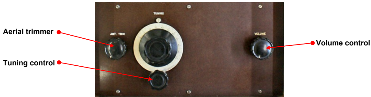
Function of controls Mk.17 receiver.
