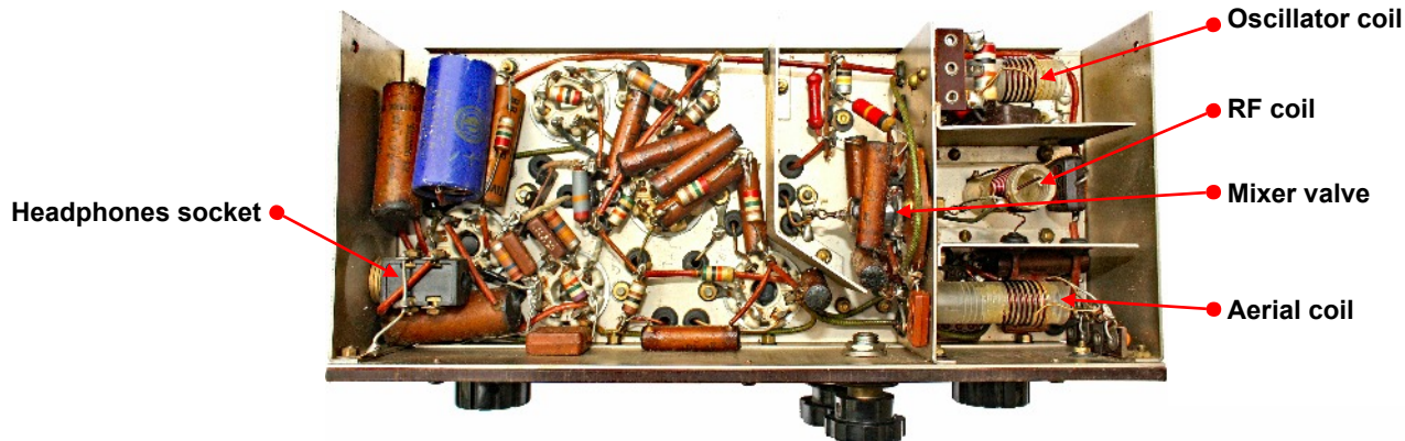
Bottom view of Mk.17 receiver chassis.
