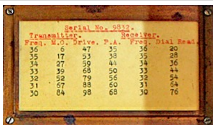
Frequency calibration card. It is interesting to note that the support/protection plate for the card is identical to that of the Mk.21.
