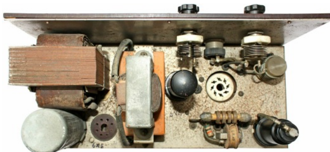
Top of chassis transmitter Mk.17. Left is the vibrator power unit with (missing 6X5) rectifier valve. On the right hand side the transmitter with 6V6 local oscillator, 6V6 RF power amplifier (valve is missing) and 6J7 modulator/pre-amplifier.
