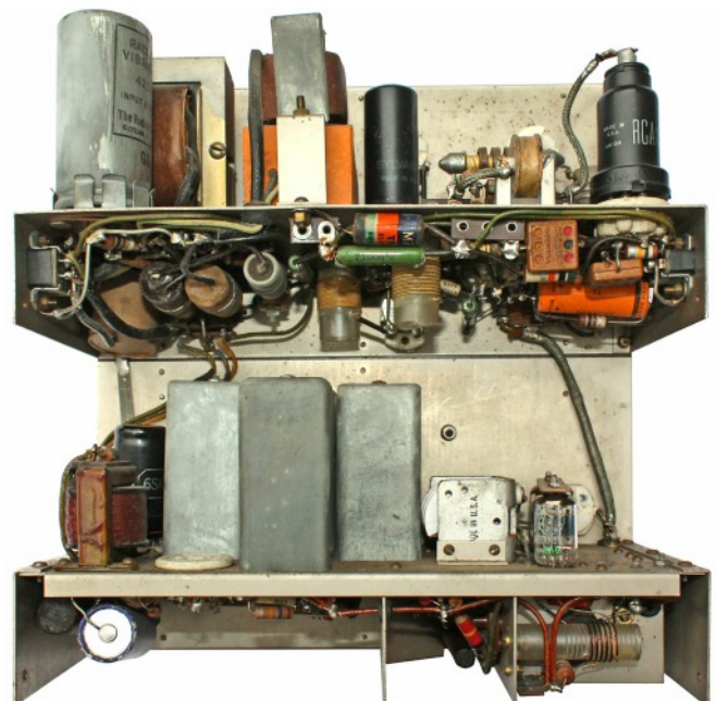
Internal view of Mk.17 showing transmitter/power unit (upper chassis) and receiver unit (lower chassis) fixed to a metal plate covered with two paxolin front plates.
