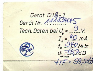
Each unit was issued with a certificate (See also Chapter 128). This 31218 certificate contain the type and serial number, DC input voltage and current, frequency, AF input sensitivity at \pm 75 kHz deviation and RF output into 50 \Omega .
