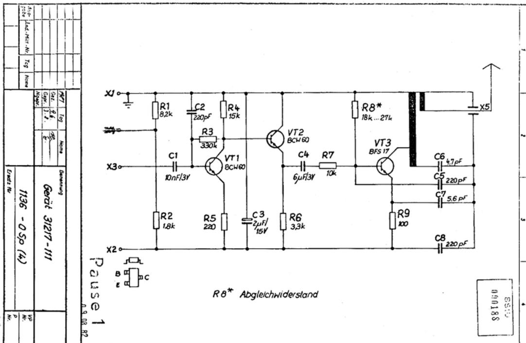
Circuit diagram of the 3127-111. This was a minor modification to the 3127-1 allowing the use of an electret microphone.
