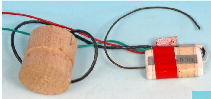
A 31217 with its microphone fitted in a wooden cylinder used for hiding in a wooden object such as the bottom of a door (left).
