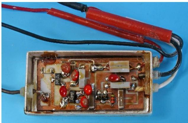
Enlarged photo of a 31217-1. The complete transmitter was mounted in a silver plated copper box, with removable lid fitted in a white plastic enclosure.
