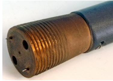
Variation of 31217-1 fitted in a tube along with batteries primarily used for overhearing conversations in the room below. The contact microphone was placed at the bottom end. The whole assembly was normally placed vertically on a wooden floor by two sharp pins fitted at the bottom.
