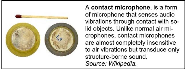
A contact microphone, is a form of microphone that senses audio vibrations through contact with solid objects. Unlike normal air microphones, contact microphones are almost completely insensitive to air vibrations but transduce only structure-borne sound.
