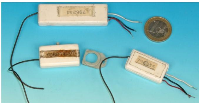
Third generation Band V bugs. Comparison of sizes between the three main standardised versions of the later Band V subminiature wireless bugs: 31218-1 (top), 31216-1 (left) and 31217-1 (right).
