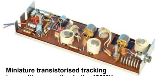
Miniature transistorised tracking transmitter operating in the 130MHz band modulated with a 1kHz tone.
