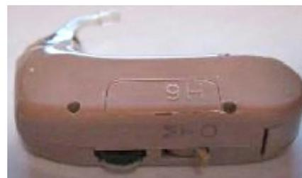
An inconspicuous wireless (induction loop principle) 'behind-the-ear' hearing aid type earphone was developed in the GDR for the PR-35 and the PR-36. It was probably imported and used in Czechoslovakia.
