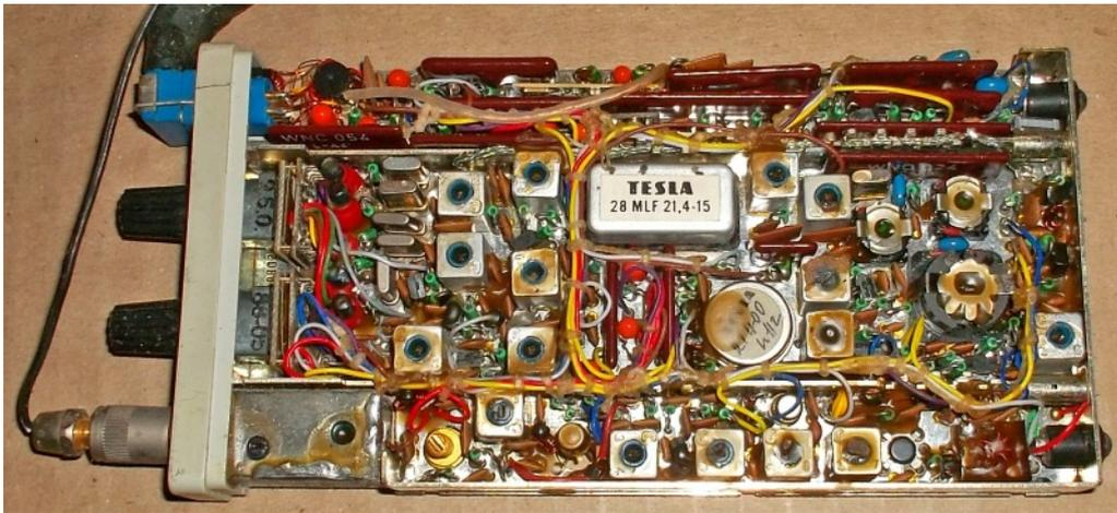
Internal view of PR-36 with its outer cover removed
