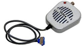
As an alternative to the miniflex aerial a wire aerial (9) was issued which could easily be concealed under the user's clothing. The red dot next to the aerial socket matched the red ring on the antenna connector. The colour red indicated the 166 MHz band, while yellow would indicate the 152 MHz band. A third colour indicated the 170 MHz band.
