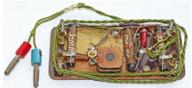
Internal view of tin cigar box midget receiver (above). Note the rectangular tuning coil and adjustable reaction coil on top. Fine tuning was by an improvised capacitor, comprising two insulated copper plates which can be seen above the coils.
