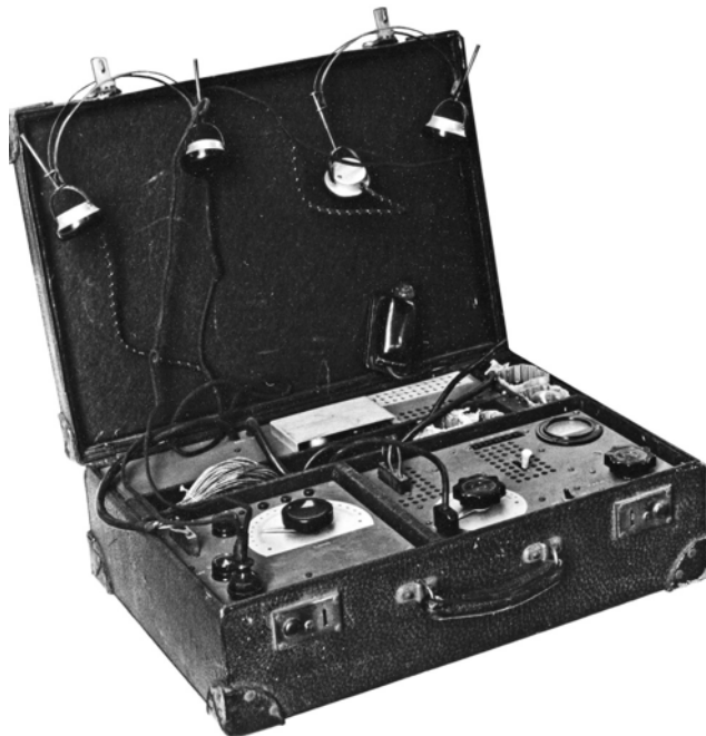
Complete SE 90/40 with power unit, accessories and spare parts packed in a suitcase
