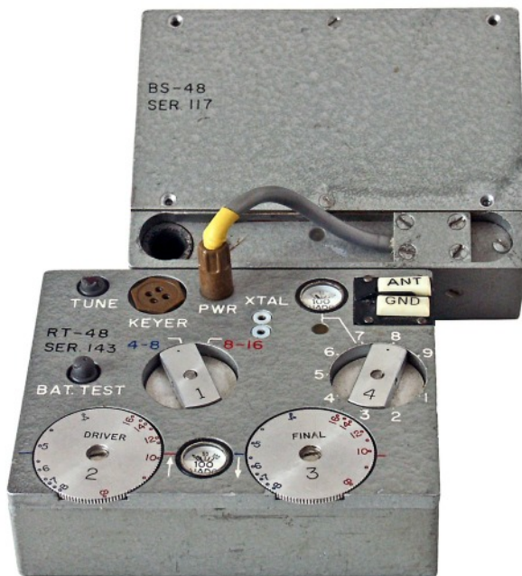
General view of a RT-48 agents transmitter with associated BS-48 battery unit.
