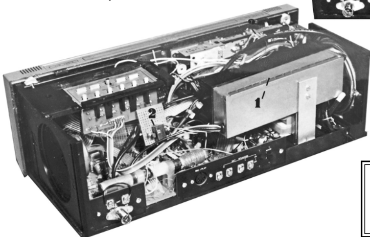
VHF transmitter hidden in a radio-cassette player/recorder with its outer case detached.
