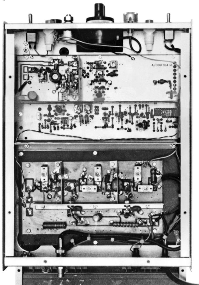
View of the oxygen controller with bottom cover plate removed showing the VHF oscillator and PLL circuit board (top); crystal controlled reference oscillator and FSK modulator circuit board (centre); driver and RF power amplifier board (below).
