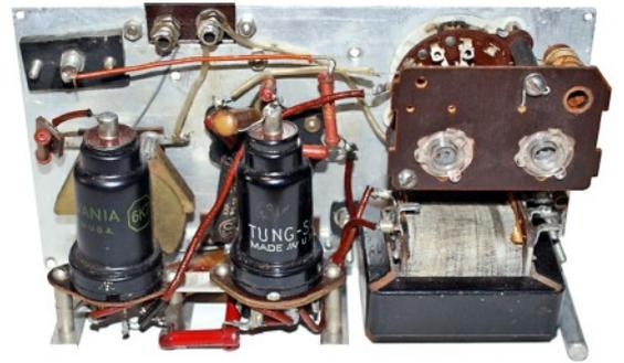
The coil block assembly appears not original, the 6.3V transformer was mounted differently, and proper valve sockets were used in this variation. This \*might\* lead to the believe to be a post war replica if not for an original Kongshavn double tuning capacitor was used.
