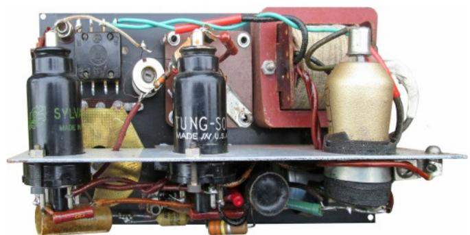
Front panel and internal view of Kongshavn variation 3. As there were no valve sockets available at the time, the valves were just wired into the circuit. Note that several components and part of the original wiring had been replaced at a much later stage.
