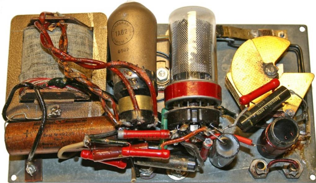
Internal view of Kongshavn variation 1. The valves were an ECH21 regenerative detector/AF amplifier and a TAB2 HT rectifier. Note the ubiquitous double tuning capacitor.
