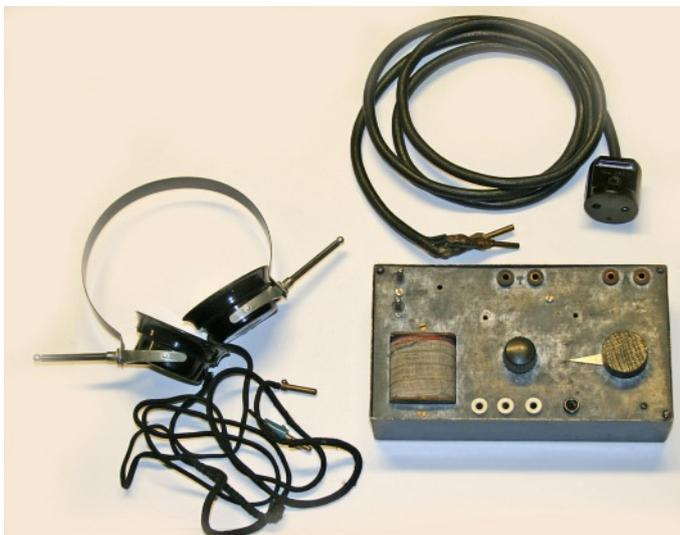
Pictured left and above is what generally believed to be one of the first produced series of Kongshavn receivers (Variation 1). Note the wooden fine tuning knob, with course tuning pointer below.
