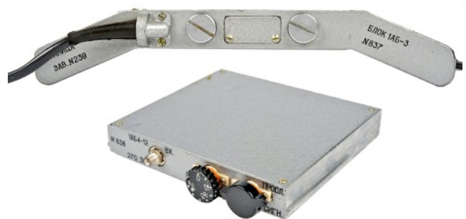
Body shaped construction of main chassis (seen from the bottom end) and one of the 12 plug-in frequency modules.
