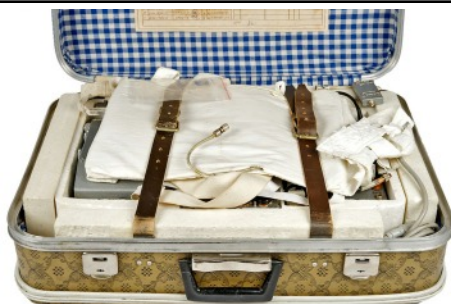
Transit suitcase for Sinitsa fully packed with body wearable cloth vest with built-in aerial on top (above), and showing all components including filters and charging arrangements (below).
