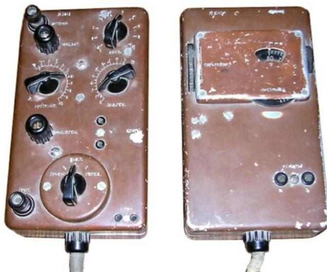
Photos of a well used Belka-4 transmitter unit (left) and receiver unit (right).
