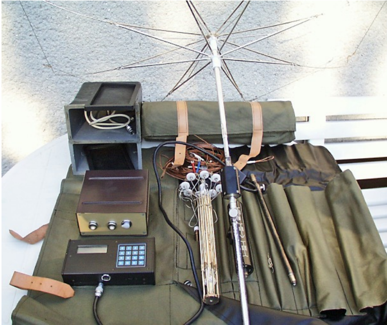
WSA 6 transmitter and high speed keyer 32843 with complete 32210-64 umbrella aerial packed in a canvas cover. (Left)
