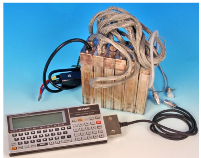
WSA 6 six-module variant for covert installation in e.g. a vehicle. A commercial Sharp PC 1600 (below) was used as control unit.
